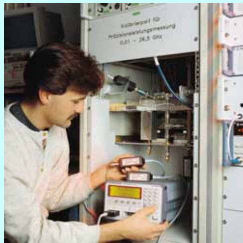
Calibration of the NRV-Z sensors is directly traceable to the standards of the German Standards Laboratory.
